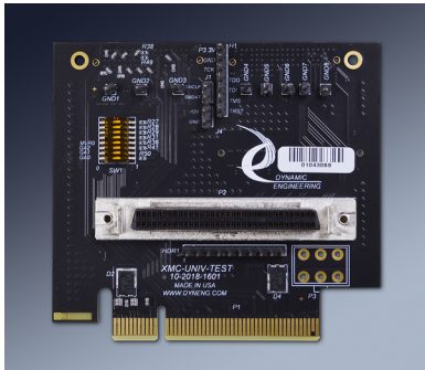
“B” Front side with the testpoints and SCSI.
