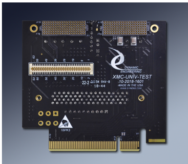
“A” Rear side with carrier type connectors to mate to XMC.
